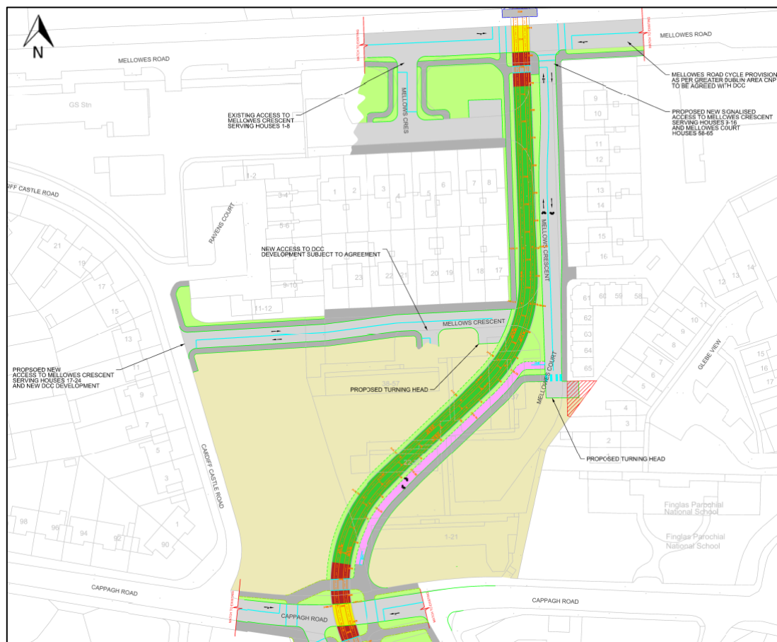
Figure 15 - Improved Micro-Option 4 (Refined Concept Design for the Luas Corridor)
