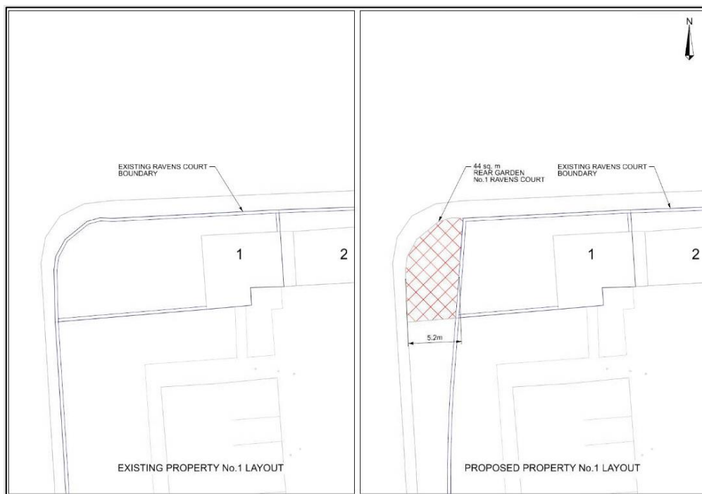
Figure 7 - Section of No. 1's garden required to accommodate the Luas corridor
