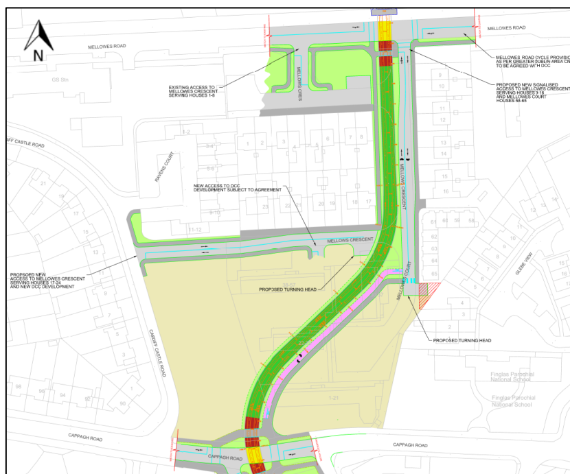
Figure 21 - Cyclist and Pedestrian Provision on Eastern Side of Luas
